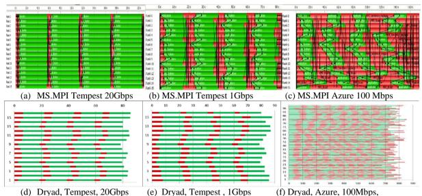
Figure 3: communication and computation pattern of 16000x 16000 PMM jobs using different runtime environments. (a) MS.MPI on 16nodes on Tempest with 20Gbps network. (b) MS.MPI on 16nodes on Tempest with 1Gbps network. (c) MS.MPI on 16 small instances on Azure with 100Mbps network. (d) Dryad on 16nodes on Tempest with 20Gbps network. (e) Dryad on 16nodes on Tempest with 1Gbps network. (f) Dryad on 100 small instances on Azure with reserved 100Mbps network.
