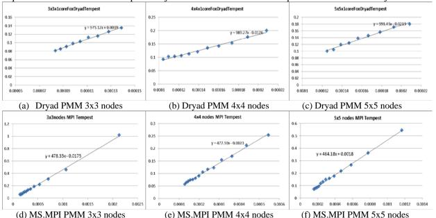
Figure 4: (a)(b)(c) plots parallel overhead vs.  $(\sqrt{N*(\sqrt{N+1})})/(4*M)$  of Dryad PMM using different number of nodes on Tempest. (d)(e)(f) plot parallel overhead vs.  $(\sqrt{N*(\sqrt{N+1})})/(4*M)$  of MS.MPI PMM on Tempest.
